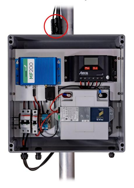
Step 12 - Insert the cable of the IDP and connect it.
