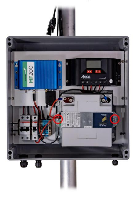
Step 9 - Connect the battery to the enclosure.
